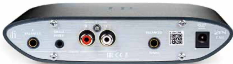
ABOVE: Powered via an external 5V wall-wart, the ZEN CAN includes balanced (4.4mm Pentaconn), single-ended (3.5mm and RCA) inputs and one balanced (4.4mm) output
